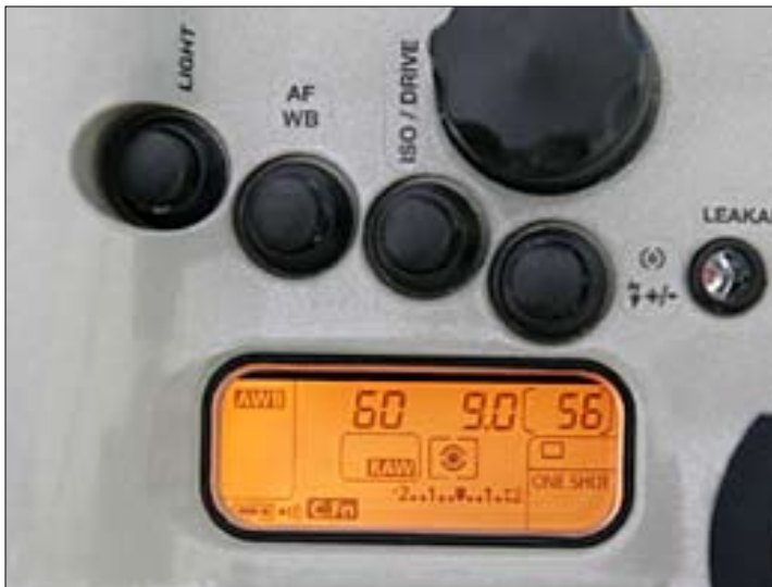
▲ The CD5's top window provides a clean view of the 5D's settings and modes.
