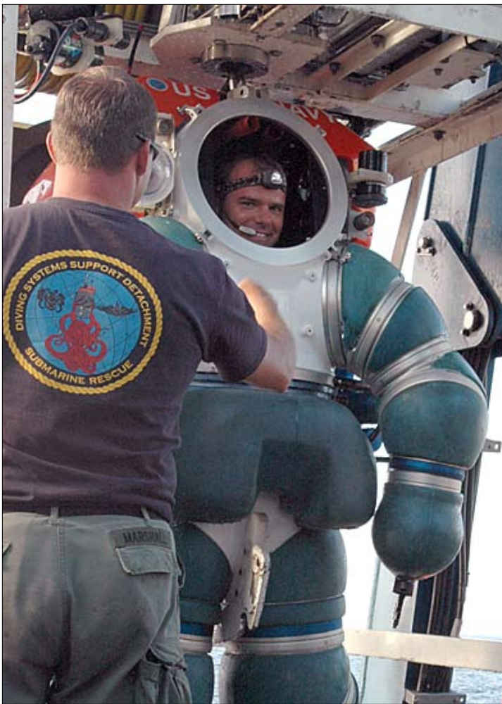
▲ Locked inside the Atmospheric Diving System (ADS) Hardsuit, Jackson eagerly awaits launch time for the first dive to be made to a target depth of 2,000 feet.
