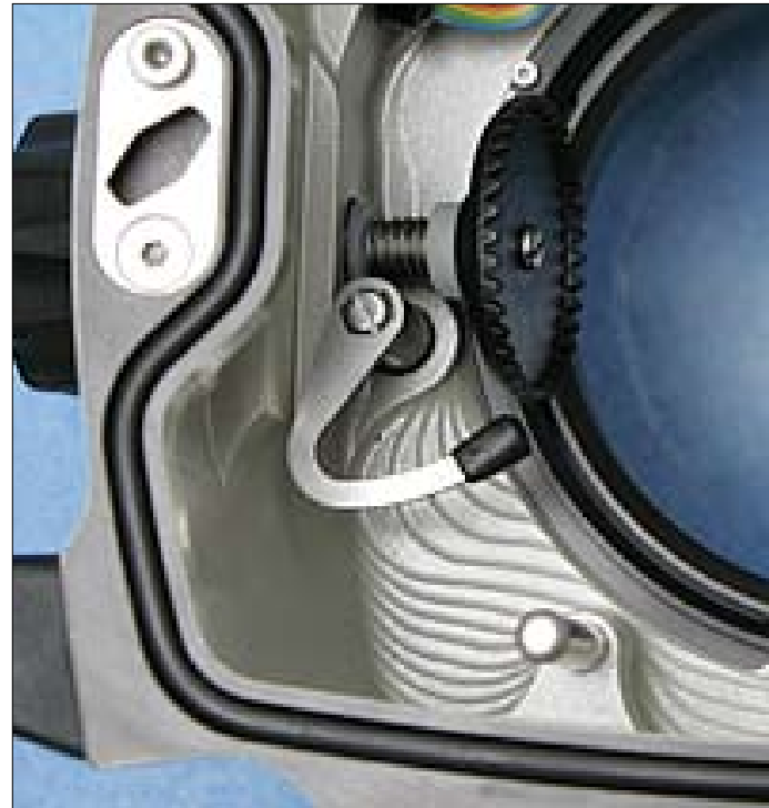
◀ This inside view of Subal's CD5 housing shows (just below the clutch for the focus/zoom gear) ingenious lever mechanism that allows the operator a simple means to depress the lens release button without removing or using the end of a pencil.
