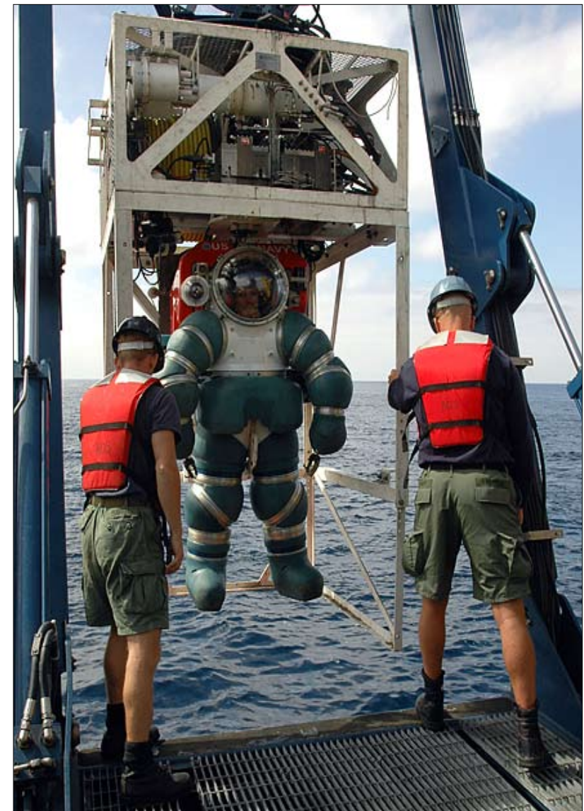
▲ Chief U.S. Navy Diver Daniel P. Jackson being launched from the M/V Kellie Chouest for the certification dive of the Atmospheric Diving System (ADS) off La Jolla, CA.
